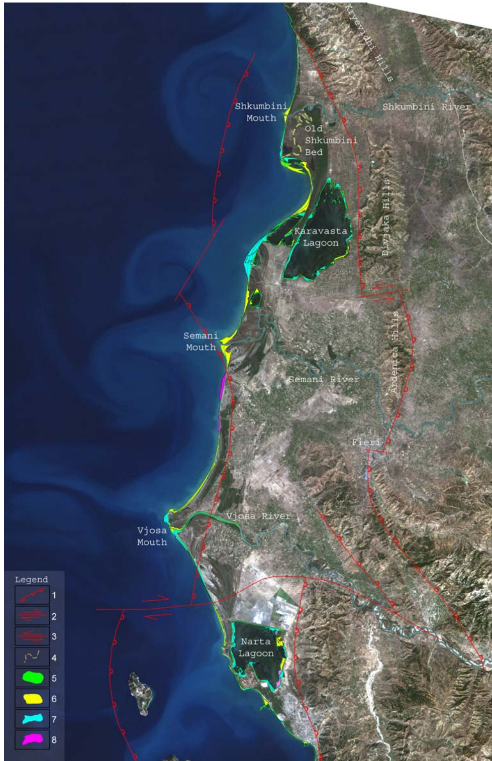
Fig. 5. Geomorphologic view of Shkumbini River-Vjosa River mouths coastline after satellite images of the period August 1981 & July 1989 & October 2001 (Global Land Cover Facility Landsat, 2005; the neotectonics active reverse faults & thrusts (after Aliaj Sh. et al. 2000).
